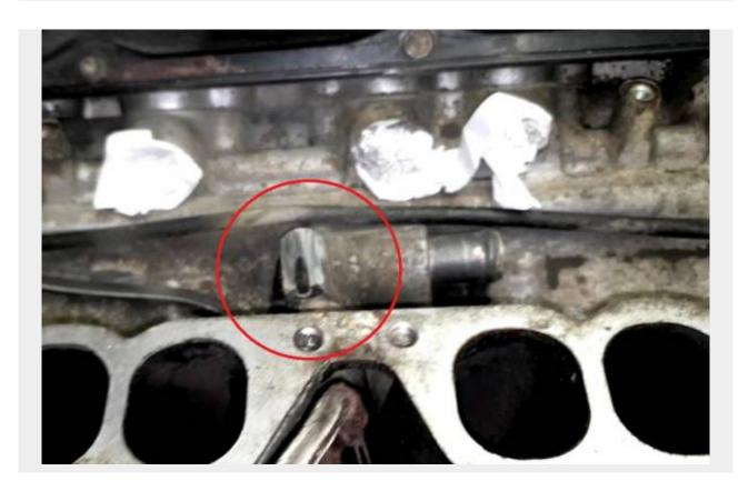
• You can plug the hole from the dispenser by screwing a metal plate with sealant to this place.
